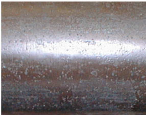
Comparison of marks left in 2 3/8" OD - 4.6 ppf 13% Cr 85 ksi Sy tubing by GRIT FACED Inserts (left) and by conventional toothed inserts (right). Unretouched digital photo at approximately 1X.
